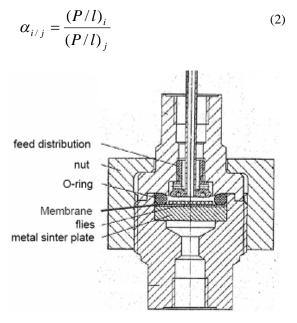
Fig. 1 Gas permeation test cell
