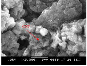
Fig. 2 FESEM image of unmodified CNTs
